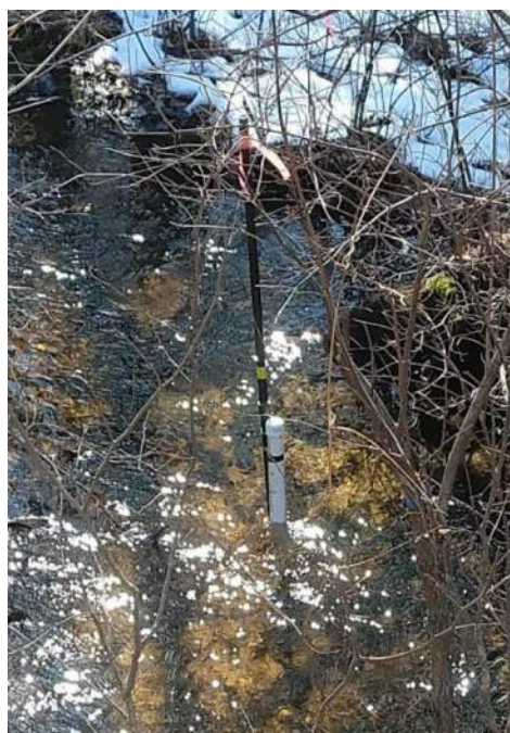
Figure 4-3: Photograph of Typical Piezometer and Stream Gauge Installation
