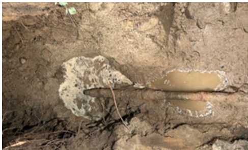
a hole in the ground with old leaking steel pipe
